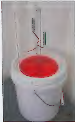
Fig. 1. Constructed light trap showing banks of LEDs and general set-up of upright clear vanes positioned over a funnel.
